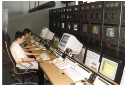
The playout control in conjunction with a self-developed automation system, completely software based and without control panels for all GVG-2100 master control switchers monitors and controls all playout activities.
