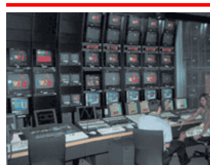
The Seven Network's presentation video system runs Thomson Saturn switchers with associated single-channel DVEs and Pinnacle Deko still stores.
