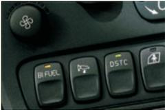
think about switching between the two fuel options (default = petrol). It is done electronically and without losing any performance while driving, but the driver has the ability to switch manually, too. The average consumption is around  $10 \text{ m}^3$  (gas) and 12 l/100km (petrol), which is for a 2.4 l engine, providing 103 kW (140 PS), not bad at all.
