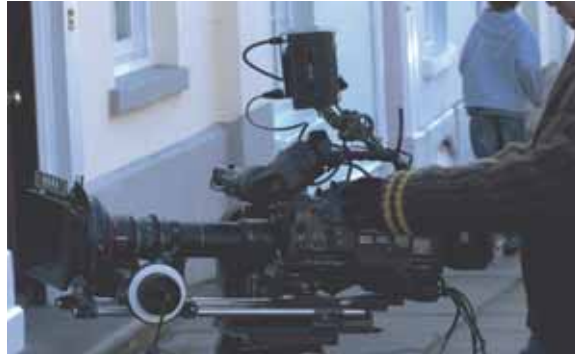
One of Canon's Prime lenses, FJ14, in action with the ACV-235 Canon Anamorphic Converter
